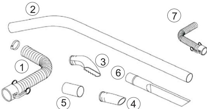
1. EPDM suction hose assembly, ø2" x 6.6' (ø50mm X 2m) female swivel camlock stainless steel AISI 316 on one end and stainless steel hose clamp on the other end..
